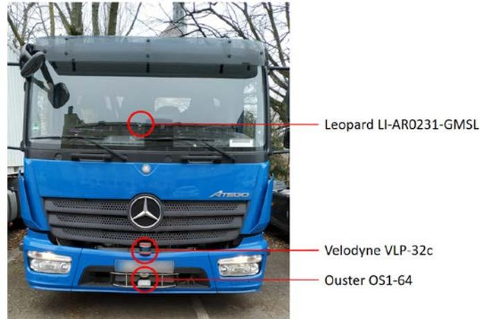
**Figure 2: Atego 823 with installed LiDAR sensors, camera and GNSS antenna**
